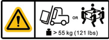
> 55 kg (121 lbs)                                                                                                            | Weight label            | The inverter needs to be carried by four persons or using a pallet truck.                                 |
